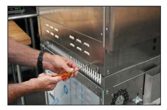
13. Secure the top unit to the bottom unit with the six bottom plate screws as shown.
