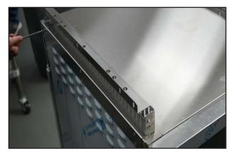
3. Locate the two side rails in the kit. Mount each rail, long side down, using the six top screws.
