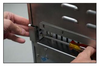
12. Insert the back trim piece in between the top unit and bottom unit. Usiing a Phillips screwdriver secure with the four provided screws.
