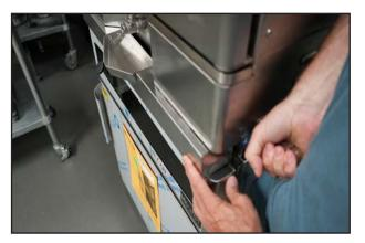
10. Place the front trim piece into place between the top unit and the bottom unit. Use a screwdriver to lift up on the top unit to properly insert the trim piece.
