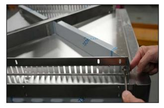
6. Locate the other short beam and mount to the long beam and the front end of the opposite side rail.
