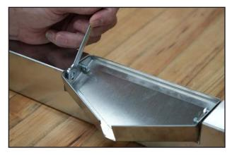
9. Locate the front drain pan and front trim piece in the kit. Using the four provided bolts and a 5/16" wrench or nutdriver, attach the drip pan as shown.
