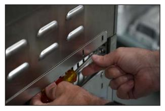
11. Secure the front trim to the side rails using the provided four screws.
