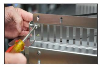
4. Locate the long cross beam in the kit. Mount as shown. Use four of the provided screws to mount to the side rails.
