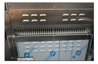
8. Align the top unit so the bottom panel screw holes are aligned with the rail holes.
