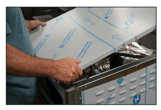
1. Using a Phillips screwdriver, remove the six top retaining screws from the unit that is going to be the bottom unit. Remove the top.
