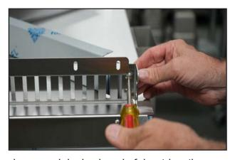
5. Locate one of the short beams and mount to the long beam and the back end of the side rail.
