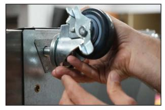
2. Locate the caster mounting holes on the drawer bottom. Carefully thread the casters into the four mounting holes. Ensure the two locking casters are in the front.
