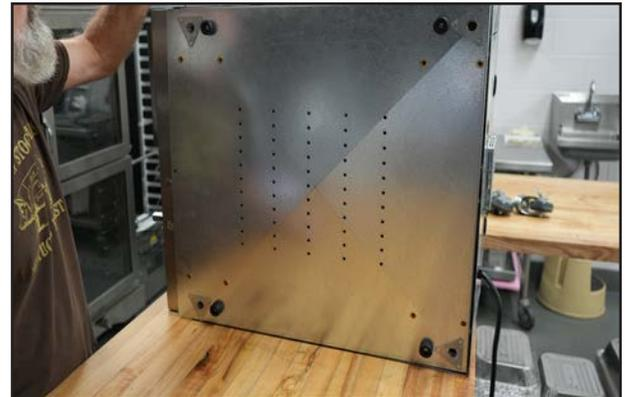
1. Remove the drawer (s). Place the unit on it's side.
