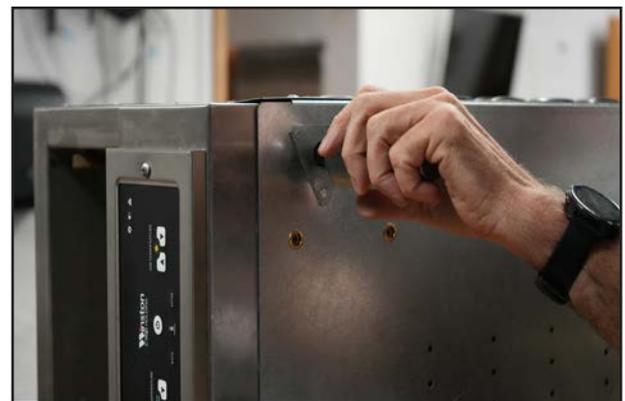
2. Locate the leg mounting holes on the drawer bottom. Carefully thread the legs into the four mounting holes.
