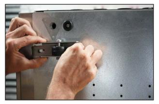
6. Ensure to tighten with the 1/8" Allen wrench. Next Install the two front wheels.
