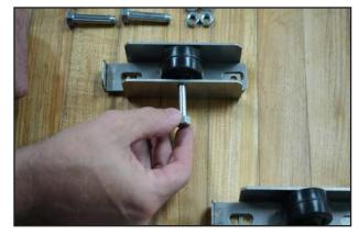
3. Set a wheel into the bracket and slide the wheel bolt through it.
