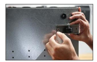
5. Locate the wheel and bracket mounting holes on the drawer bottom. Start with the back wheels. Using the provided screws and an 1/8" Allen wrench mount the two back wheels.
