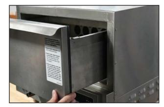
8. Verify that the locks slide back and lock the wheels into place. Replace the unit drawer
