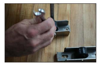
4. Thread on the wheel nut and tighten using two 1/2" wrenches. Repeat the process with the other front wheel and the two back wheels The back wheels will not have a locking plate.
