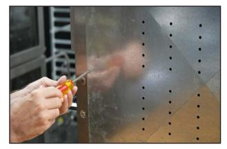
6. Insert the new bottom into place. Verify that the bottom screw hole is towards the front. Replace the bottom screw.
