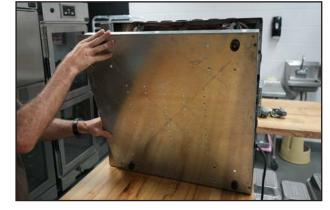
5. Remove the screw from the drawer bottom. Remove the drawer bottom.
