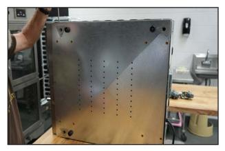
7. Replace the topside screws and the backside screws.
