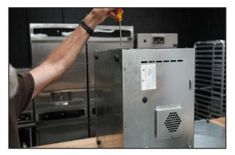
4. Remove the three screws from the topside bottom.
