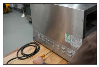
1. Remove the drawer (s). Remove the three screws from the bottom of one side of the drawer unit.
