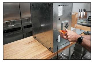
3. Remove the three screws from the bottom back.
