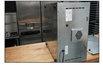
2. Set the unit on the side where the three screws were removed.
