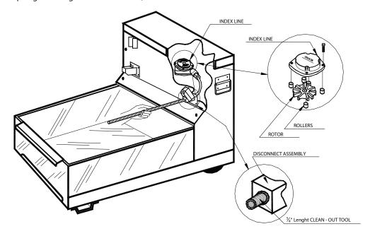
3. Remove spring; plug in power cord; turn on pump. Make sure connected hoses are cleared of solidified shortening.
