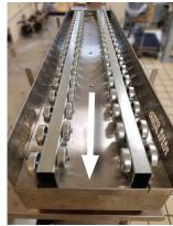
3. Secure the conveyor to the top of the oven using the suction cups under each end. This prevents the conveyor from sliding.
