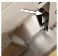
4. Insert the bubble fork into the two provided hooks.
