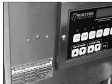
View of fryer after new high limit thermostat is mounted.
