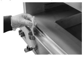
8. Inspect heating elements (if exposed). The elements are stainless steel. If cleaning is needed, scrub with Teflon™ or nylon bristle brush to remove heavy food particles. Further cleaning may be done with a plastic scouring pad and alkaline based cleansers. DO NOT use wire brushes, scrapers, steel wool pads or chloride-based cleansers. Follow cleanser manufacturer's instructions for use on stainless steel. Rinse well with clean water and wipe immediately.
