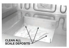
6. Wipe down all outside surfaces with mild detergent, in particular where the drawer seals. Also clean the gasket. This procedure will prolong gasket life.
